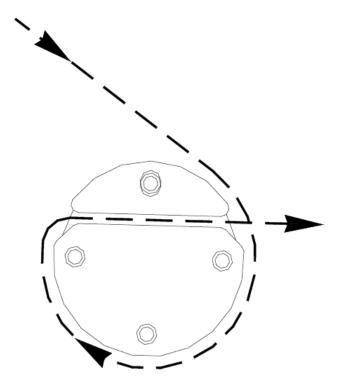
To install the string, wrap the string around the drum in a clockwise direction. The string should pass over the top of the drum and then back between the jaws of the drum. Before rotating the drum, pull the string slightly to remove excess string.
